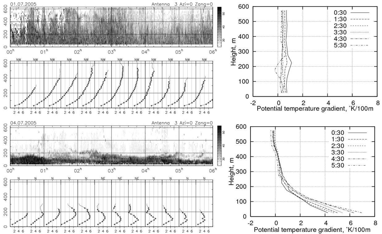
**Figure 2.** Echograms of acoustic sounding and wind speed profiles (left panel) measured by LATAN-3 sodar and profiles of potential temperature gradient (right panel) in night-time for those dates as in Fig.1. Gray scale on echograms is proportional of scattering intensity ( $C_T^2$ ) in logarithmic units (shown on the right side). On the left side height is shown, below echograms LST is pointed, below wind profiles scale of wind speed is displayed as well as direction is shown above
