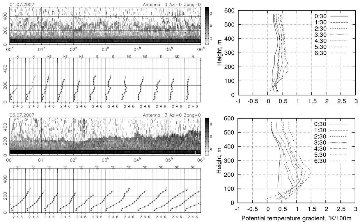
**Figure 7.** Comparison of echograms and wind profiles in centre of Moscow for weak and strong wind speed. At the right panels profiles of PTG are displayed.
