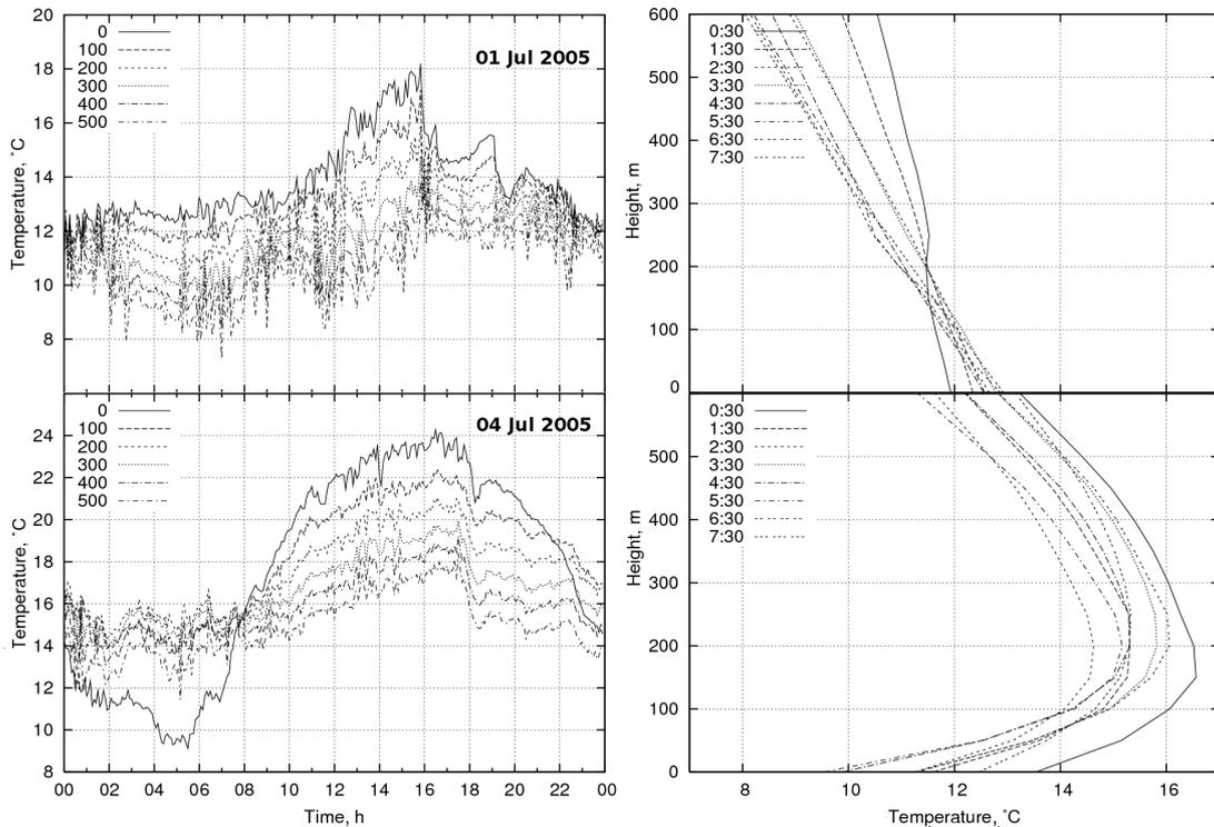
**Figure 1.** Diurnal course of temperature at different heights (left panel) and profiles of temperature averaged over 30 min in night-time (right panel) measured by MTP-5 profiler at rural area (ZSS of IAPh) for two cases of night ABL stability: weak ( 01 July 2005, above) and strong (04 July 2005, below).
