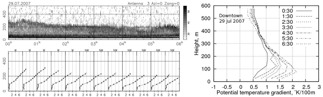
**Figure 5.** Comparison of MH by sodar echograms and PTG by profiler measurements for vary stable situation in urban area. (Explication is shown in Fig. 2)
